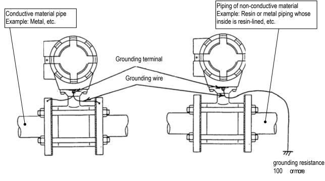
• If the piping material is conductive, connect the grounding wires to the both ends of the piping flange. • If the piping material is non-conductive, perform grounding (grounding resistance 100 or less).
